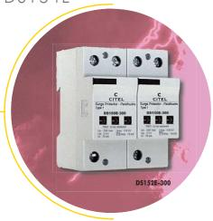
DS150E AC surge protectors are designed to be connected in multi-pole configuration to protect single phase, 3-phase and 3-phase+Neutral AC networks. They are sometimes associated with a dedicated N/PE SPD (DS100EG, «Gas tube» technology surge protector).
