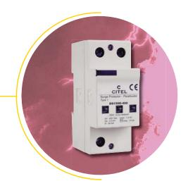
The DS150E is a Heavy Duty Type 1 AC Surge Protector Device (SPD) designed to be connected at the entrance of the electrical installation. This SPD provides an efficient protection against direct and indirect effects and is particularly useful in a high lightning density area where the risk of heavy surge current or even direct strike is high (e.g.: buildings equipped with lightning rods).
