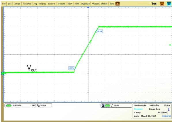
Figure 15: Startup by power-on
