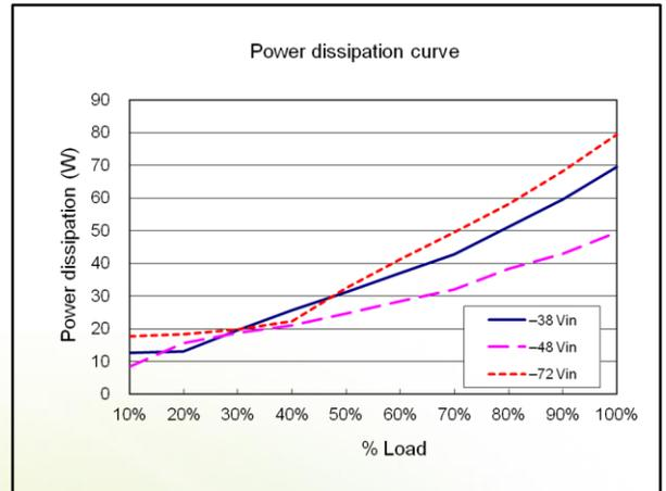
Figure 2: Power dissipation ( $T_A = 25^\circ C$ ,  $V_{out} = -54 V$ )
