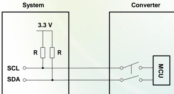
Figure 21: Interconnect diagram of SCL and SDA
