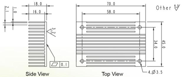
Figure 27: Standard heat sink for airflow from  $V_{in}$  to  $V_{out}$
