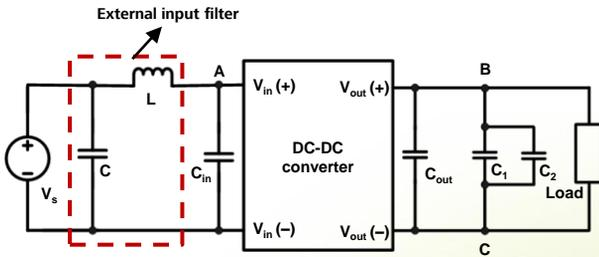
Figure 7: Test set-up diagram
