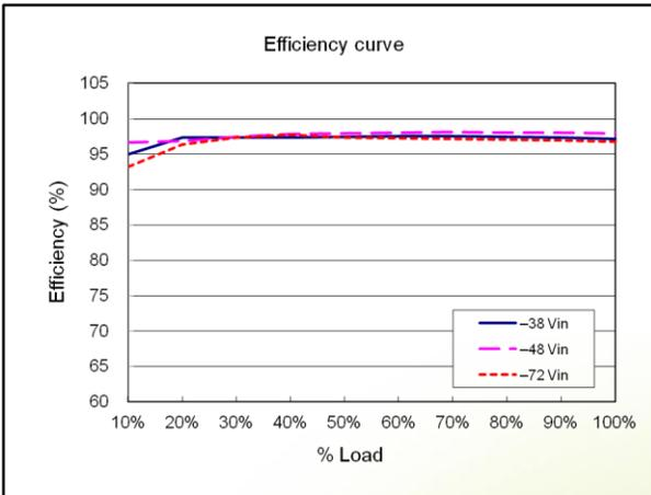
Figure 1: Efficiency ( $T_A = 25^\circ C$ ,  $V_{out} = -54 V$ )
