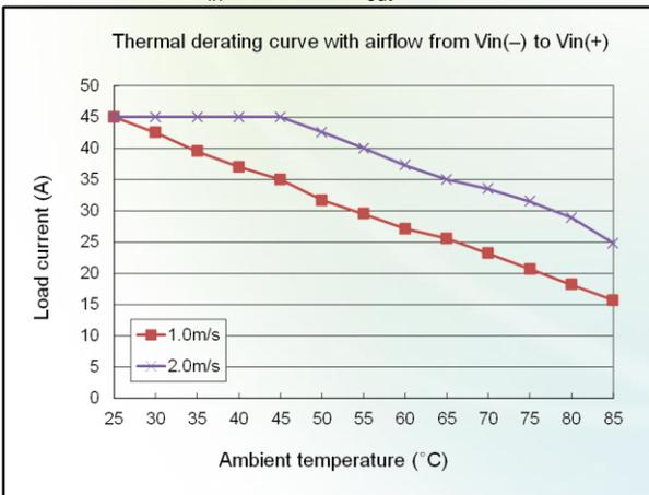
Figure 5: Thermal derating with airflow from Vin (-) to Vin (+) ( $V_{in} = -60 V$ ,  $V_{out} = -54 V$ )
