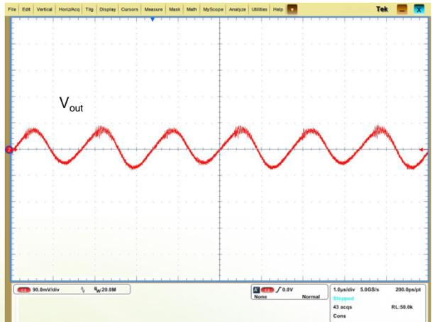
Figure 10: Output voltage ripple
