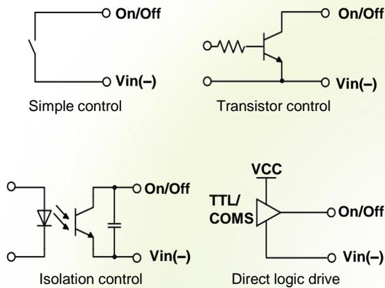
Figure 20: Various circuits for driving the On/Off pin
