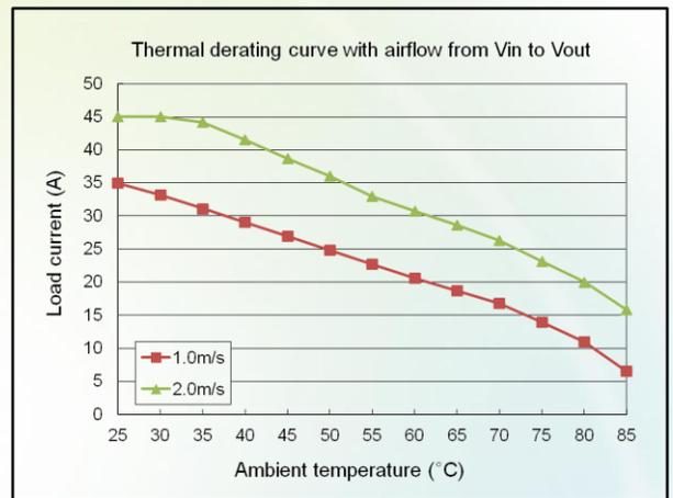
Figure 4: Thermal derating with airflow from Vin to Vout ( $V_{in} = -48 V$ ,  $V_{out} = -54 V$ )
