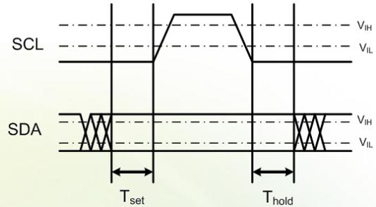
Figure 22: PMBus setup time and hold-up time
