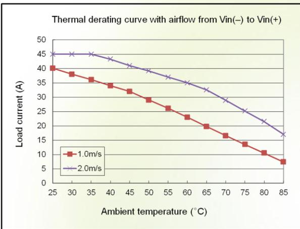
Figure 3: Thermal derating with airflow from Vin (-) to Vin (+) ( $V_{in} = -48 V$ ,  $V_{out} = -54 V$ )
