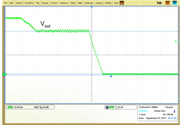
Figure 16: Shutdown from On/Off
