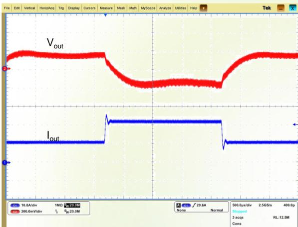
Figure 17: Output voltage dynamic response
