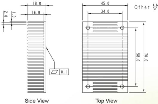
Figure 26: Standard heat sink for airflow from  $V_{in}(-)$  to  $V_{in}(+)$
