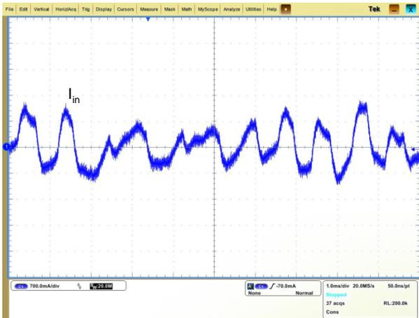
Figure 9: Input reflected ripple current
