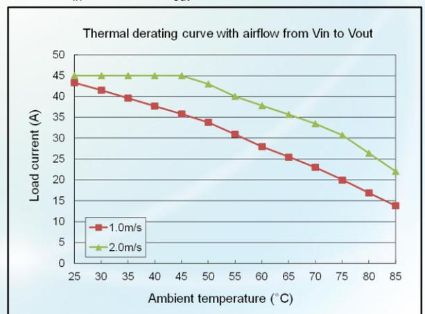
Figure 6: Thermal derating with airflow from Vin to Vout ( $V_{in} = -60 V$ ,  $V_{out} = -54 V$ )
